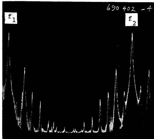
Fig. 3. Spectrogram of small full-range direct radiator employing several small cone loudspeaker elements and a pre-amplifier equalizer. First peak f_1 = 50 Hz, followed by a small 2f_1 component, and 3f_1 , 4f_1 , etc. Second large peak, f_2 = 750 Hz, flanked by small first-order sidebands of f_2 \pm f_1 and larger sidebands of f_2 \pm 2f_1 , and significant third- and fourth-order sideband frequencies. Total modulation distortion, approximately 14%. Input of both frequencies adjusted to produce 95 dB SPL at 2 ft.
